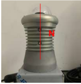
Figure 20 – A picture showing how to correctly orient the all-sky camera of the StAnD Meteor Camera Kit to the North. The camera protective case has two bolts vertically arranged showing outwards (marked with the red line on the picture), with which the camera module is fixed to the inside of the case itself. Due to the internal arrangement of the components, the bottom portion of the CMOS is always facing this direction. Therefore, if one aligns such direction towards the North, an approximate reference frame can be defined a priori, and all cameras of the network can have the same approximate orientation.
