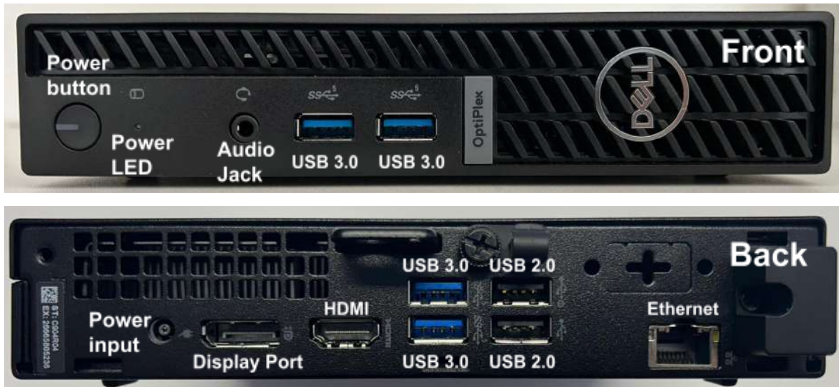
Figure 12 – Pictures of the front (top panel) and back portion (bottom panel) of the Mini-PC with ports and buttons highlighted.
