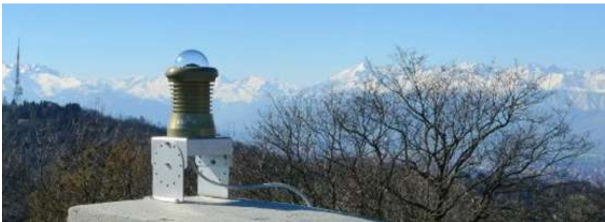
Figure 1 – The first all-sky camera of the PRISMA network in Italy, installed in 2016 on the roof of the office building of the Astrophysical Observatory of Torino, part of INAF - the National Institute of Astrophysics.
