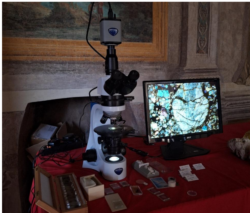
Figure 12 – In this photo, the microscope is connected to a monitor showing a chondrule
